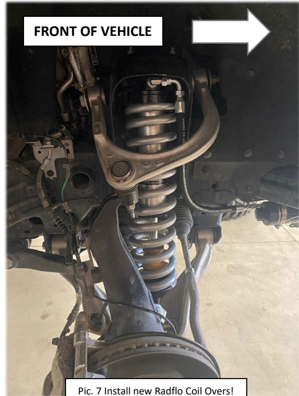
Pic. 7 Install new Radflo Coil Overs!
