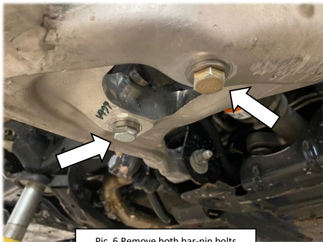
Pic. 6 Remove both bar-pin bolts from the lower control arm.
