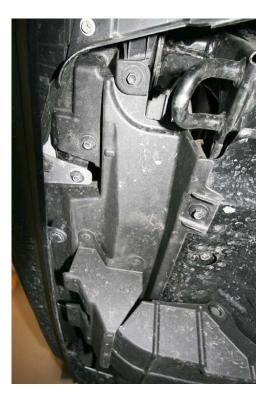
3. Remove plastic air scoop from skid plate (if fitted). Pull out the center of the large plugs before removing them.
