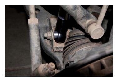
16. Insert the lower bolt and tighten the nut. Reverse of step 7. Torque the lower bolt to **75 ft/lb**. Tip:- Push down on the upper control arm with a pry bar to make it easier to line up the coilover hole with the lower mount and bolt.
