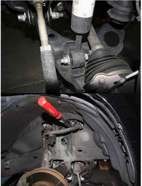
11. Remove the 3 top bolts holding the strut assembly to the frame.
