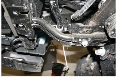
6. Remove the swaybar end link nut and swaybar link from the spindles on each side. Let the links hang loose from the spindle. **Tip:-** If the nut simply rotates the bolt on the ball joint, insert a metric allen wrench to the end of the bolt to hold it in place.
