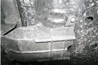
4. Remove the 4 bolts retaining the front skid plate. Then remove skid plate.
