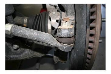
9. Use a tie rod puller to separate the tie rod form the spindle. Be careful not to damage the rubber boot on the tie rod. Once separated move the steering link away from the spindle to allow more space to remove the strut assembly later.
