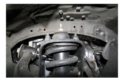
12. Push down on the upper control arm with a pry bar while moving the strut out of the lower mount and down slightly. Then slide it out towards the front while releasing the pry bar and moving it out underneath the upper control arm.
