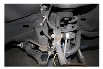
7. Now undo the bolts holding the swaybar bushing brackets and then remove the swaybar from the vehicle. **Tip:-** The front 2 holes on the bracket are open allowing you to slide the bracket out. Thus remove the 2 bolts to the rear and then undo the 2 front, but don't remove. Then simple slide the bracket and swaybar out towards the rear.
