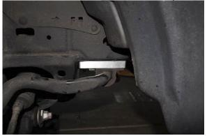
20. Insert the swaybar end link bolts through the spindle holes. Reverse of step 3. Torque the nuts to **52 ft/lb**.
