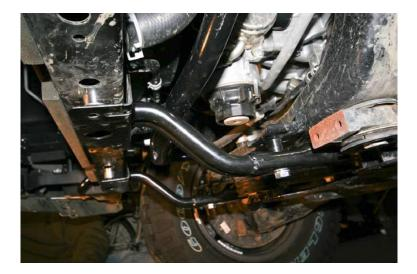
22. Install the front skid plate. Note that the tabs on the front will no longer fit in the frame. Do not over tighten the bolts and strip the threads.
