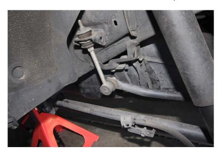
3. Undo and remove the lower shock absorber bolts.
