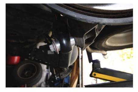
9. Tighten the top shock absorber mount nuts. . Please note the following when installing your Radflo shocks product with a pin mount on the end cap (generally the top of the shock):
