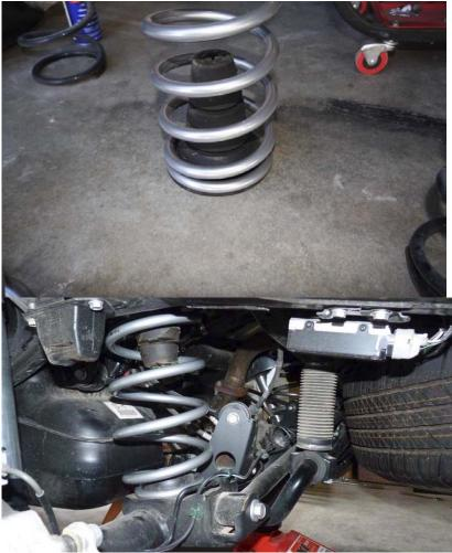
7. Install the new rear shock absorbers by first inserting the top bolt. Make sure a bushing and washer is on both sides of the frame mount. Do not tighten the top mount at this time.
