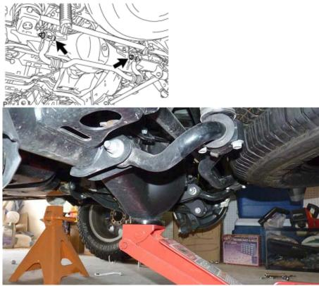
3. Undo and remove the lower shock absorber bolts.
