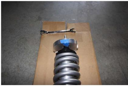
9. Tighten the top 3 bolts. Make sure to use the supplied washers. Hand/wrench tight only.
