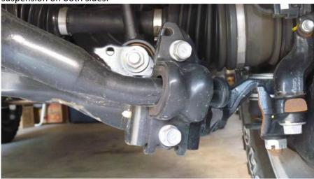
3. Undo the cotter pin in the steering outer tie rod end and then remove the castle nut.
