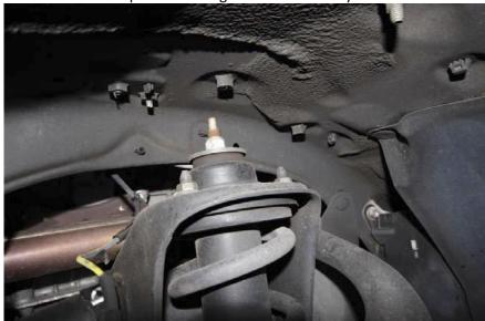
7. Push down on the upper control arm with a pry bar while moving the strut out of the lower mount and down slightly. Then slide it out towards the front while releasing the pry bar and moving it out underneath the upper control arm. **Tip:-** Move the swaybar out of the way of the coilover when sliding it past the lower control arm.
