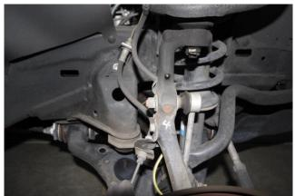
4. Now undo the bolts holding the swaybar bushing brackets and then remove the swaybar from the vehicle. **Tip:-** The front 2 holes on the bracket are open allowing you to slide the bracket out. Thus remove the 2 bolts to the rear and then undo the 2 front, but don't remove. Then simple slide the bracket and swaybar out towards the rear.
