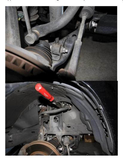
8. Remove the 3 top bolts holding the strut assembly to the frame.
