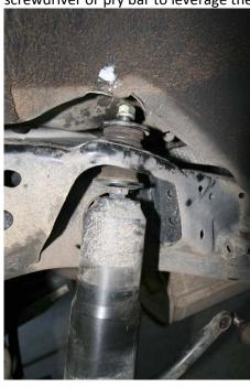
5. Droop the rear axle and remove the rear coilsprings. Push the springs up and remove from lower bucket and then pull the springs towards the rear and outer axle to remove from vehicle. **Tip:-** On some vehicles the rear axle might have to be pushed down to allow more room for removal of springs.
