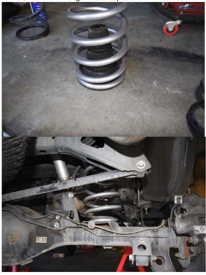
7. Install the new rear shock absorbers by first inserting the top bolt. Make sure a bushing and washer is on both sides of the frame mount. Do not tighten the top mount at this time.
